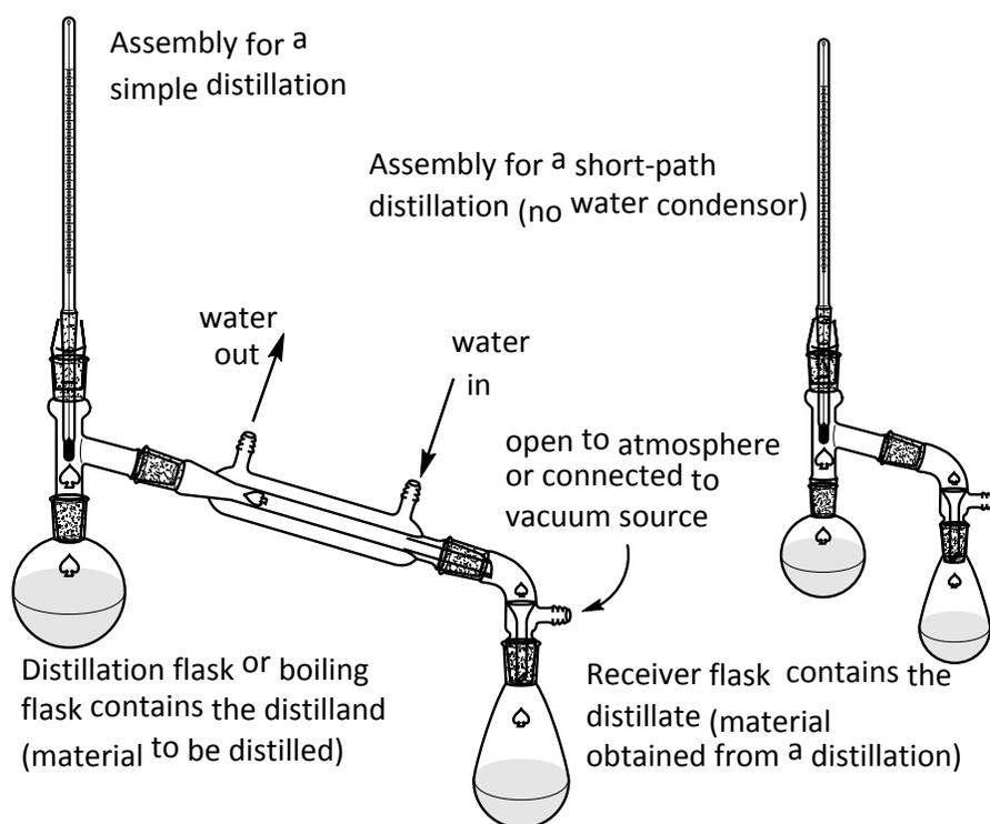
The first compound to distill, acetone, is a relatively harmless substance. However acetone is flammable so open flames will not be used. A hot water bath will suffice as a heat source. Acetone is a compound with high vapor pressure; it is volatile meaning it evaporates readily at room temperature. A typical set-up is shown here.
