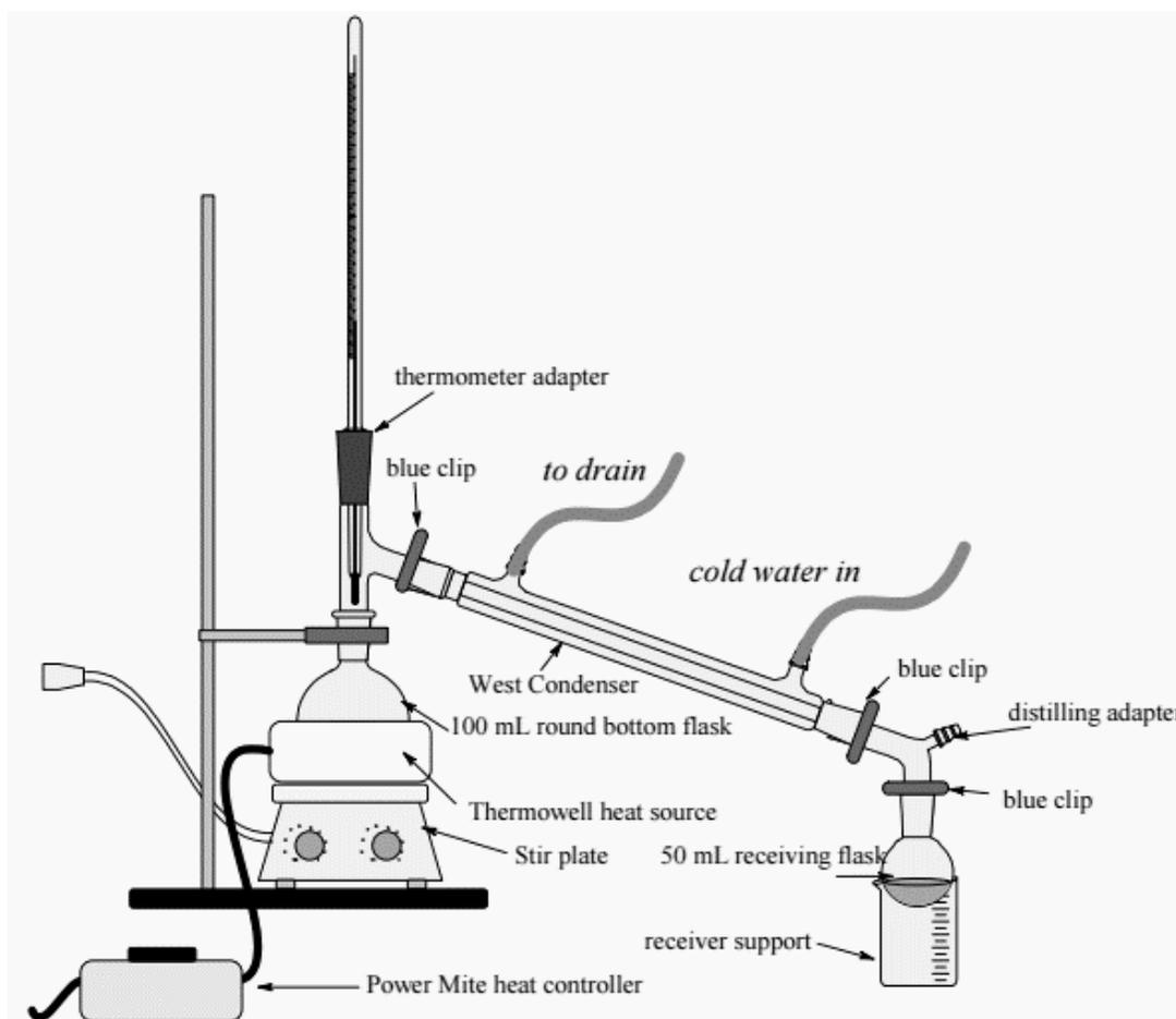
Plastic clips can be used to connect glass joints that will not be in contact with excessive heat. Otherwise, the wire spring clips can be used.
